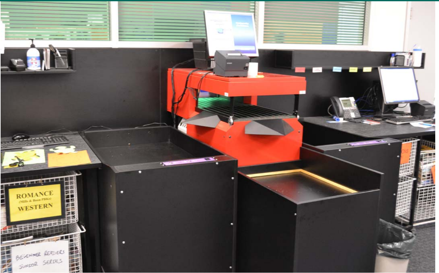
Compact sorter with three bin sort - E.M. or RFID controlled.
